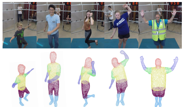
Figure 5: We reconstruct the body occupancy map and its outer surface using shape-from-silhouette and associate the point cloud with body semantics (head, body, arms, and legs).
